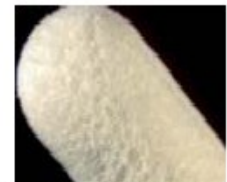
UltraSOLV® Tip After HSA Swabbing
